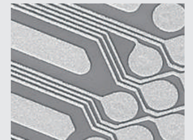
▲ Enlarged view of inner layer wiring for data center
