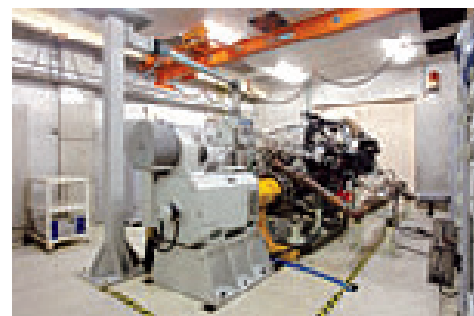
Performance evaluation of SiC-DPFs with engine bench test We are updating the engine and evaluation system to meet the latest exhaust emission regulations.
