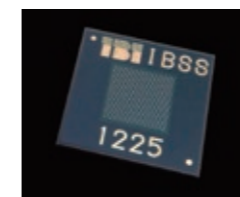
5 IC Package Substrate (1988-present)
